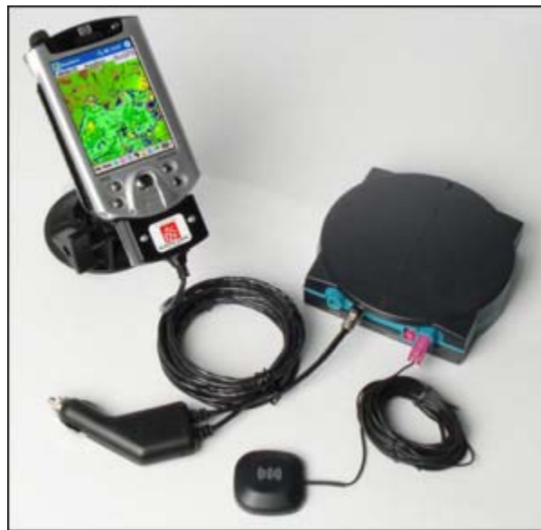
Clockwise from top: HP iPAQ 5500; Wx Worx satellite receiver; Receiver antenna; PDA/Receiver power supply; System includes Anywhere Bluetooth® wireless GPS (not shown).
